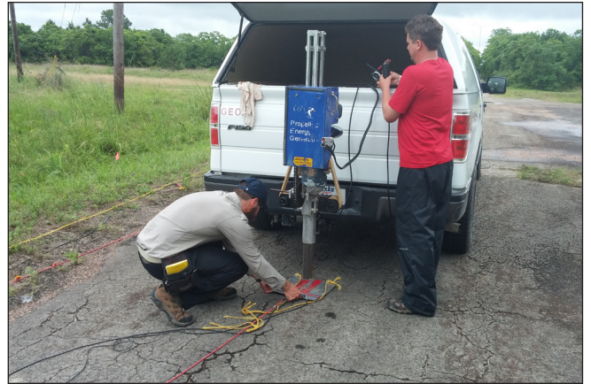
Figure 3: Students work together to set up a source for near surface seismic using a wacker. Photo by Jyl Verner
